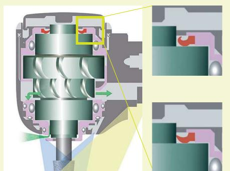
During rotation, the uniquely designed rubber brake ring in TwinPower is pulled away from the turbine axis.
